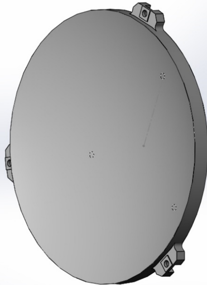
Figure 1: Resulting 6.00" diameter (152 mm) concave spherical test mirror design. All interferometric testing was conducted when resting face up in a free state of constraint for vertical testing or mounted for horizontal testing under light fastening spring pressure to the three raised pads on the back side.
