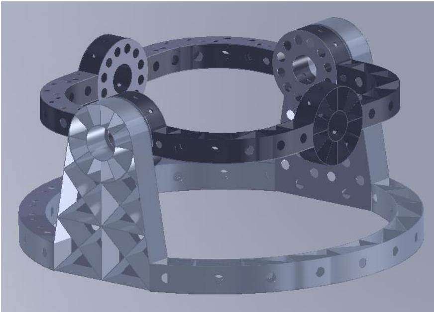
**Figure 1:** The top view shows the notional gimbal with 300 mm aperture, 10 Kg dummy payload and light weighted and skinned over pocket structure. The bottom view illustrates interior views with the skin removed in some areas to illustrate the rib structure. An all solid design with identical outside dimensions was also modeled for comparison
