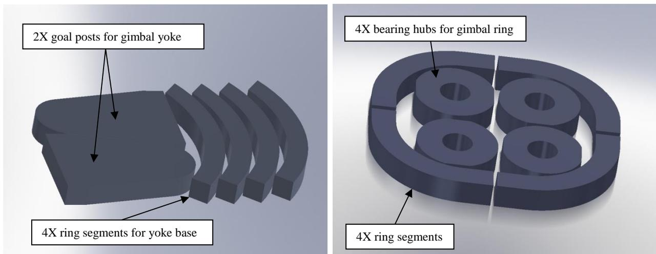
**Figure 3:** The gimbal yoke (left) and gimbal ring (right) can be efficiently manufactured from blocks of beryllium or aluminum-beryllium material by slicing out the parts, including skin pieces and interior pockets by wire EDM, then brazing or welding all of the parts back together. Individual parts can also be cast or near net shaped prior to final machining and brazing or welding.
