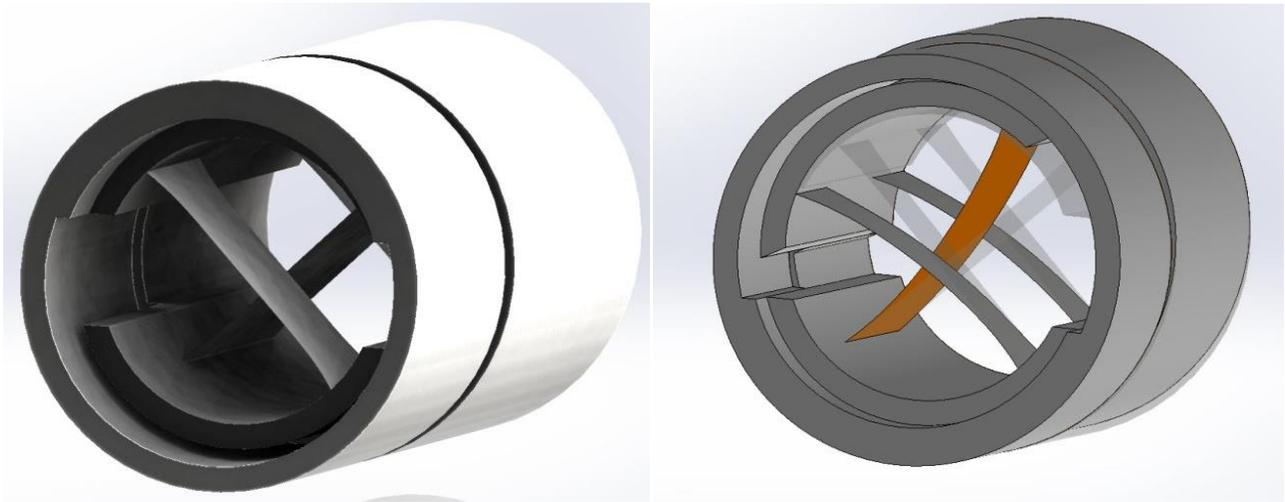
**Figure 4:** A Bendix type rotary flexure shown in a free state of constraint on the left and after simulation of rotation at the right. Non-linear FEA methods were used to compare the virtual performance of 420 stainless steel to an amorphous metal alloy produced by Light Metals Technologies.
