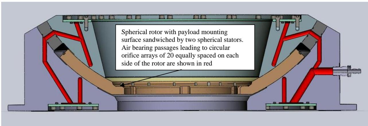
**Figure 6:** Many configurations of spherical gas bearing gimbal designs have been developed. The above figure illustrates the cross sectional view of a large spherical air bearing gimbal developed as a part of a simulation system. The system provides virtually frictionless motion in three axes and a large load capacity.
