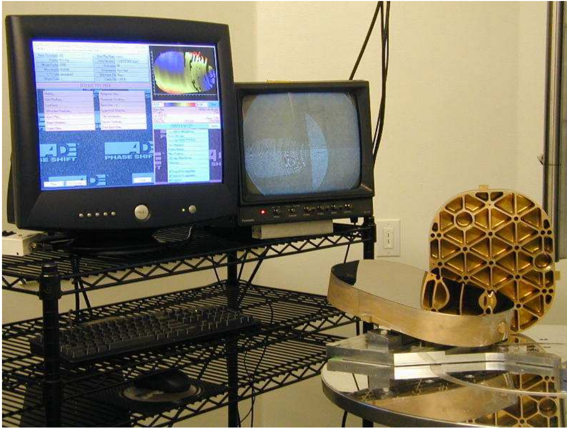
Figure 4: This photo shows a 15" aperture, light-weighted, nickel plated aluminum mirror that is an off-axis segment of a 38" diameter general case aspheric surface of revolution. This mirror is the tertiary mirror for a four-mirror, off-axis variable zoom system. The iso-grid light-weighting structure typical of all of the mirrors can be seen in the primary mirror in the background. The tertiary mirror is null tested for optical polishing utilizing a CGH and on-process, vertical axis, phase measuring interferometry. Since the mirror exceeded the 12" radial tool travel of the diamond turning machine, it's surface was blended with two cuts both before and after nickel plating to produce a near-net optical figure of about 2.0 waves RMS @632.8 nm and 150 Angstroms RMS surface finish. Electroless nickel plating was also held to less than 0.0015" to minimize the potential for bi-metallic distortion over the operational temperature range. The mounting geometry was thrown off in tilt by centrifugal turning forces and unsymmetrical mounting by 0.001" in the circumferential direction and 0.0025" in the radial direction. Mounting geometry is then corrected to within 0.0002" tilt over the mirror overall dimensions, figure is corrected to less than 0.10 wave RMS @632.8 nm, and surface roughness is improved to less than 30 Angstroms RMS with all artifacts of diamond machining periodic structure erased.
