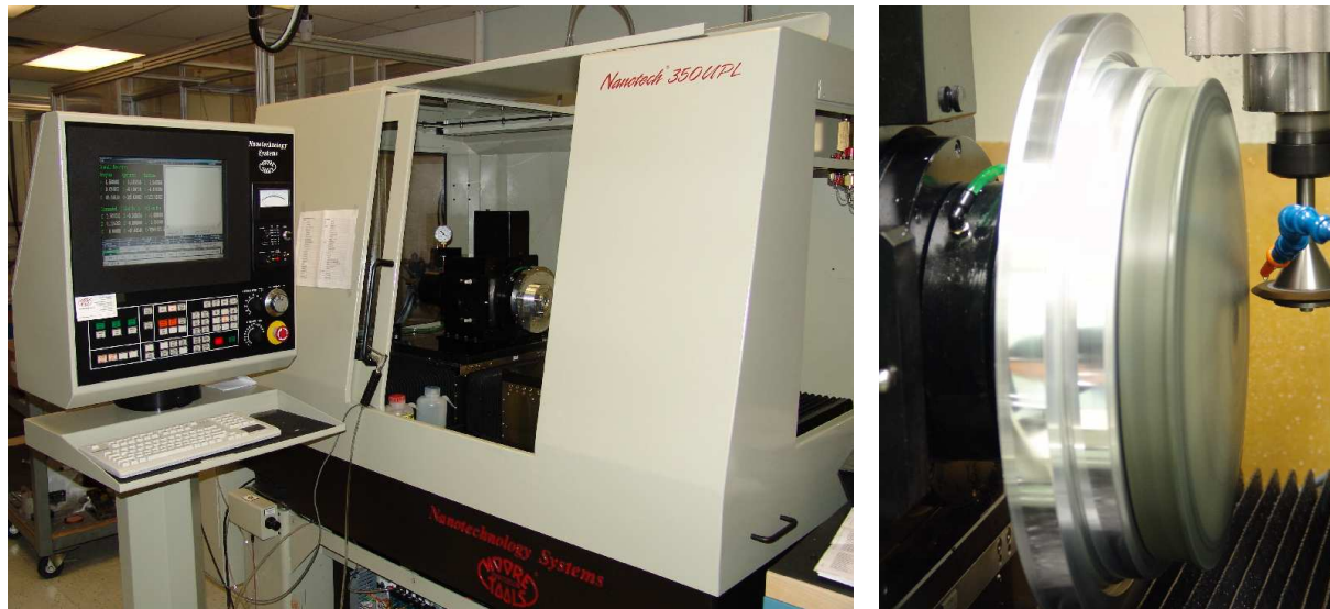
Figures 2: Left photo shows a state-of-the-art diamond turning and grinding machine. The right photo shows a 290 mm light weight CVD SiC clad SiC mirror undergoing hard wheel aspheric grinding prior to computer polishing. The optical figure from grinding was about 2.0 waves P-V @632.8nm and less than 50 Angstroms RMS surface finish; ideal initial conditions from which to commence computer polishing. “Slow tool servo” capability and on-machine profilometric measurement technologies also provide the means to fabricate and measure complex aspheric surfaces including those not having rotational symmetry with the machine axis.
