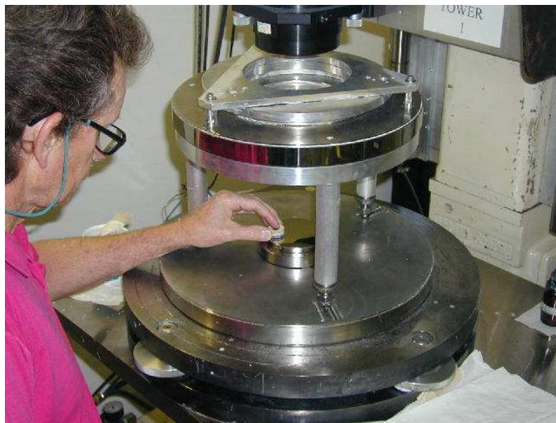
Figures 3: The photo at left depicts a large, off-axis, general aspheric, nickel plated and post polished aluminum mirror tested in the presence of a computer generated hologram (CGH) and phase measuring interferometer. The optical axis of the null test is precisely registered to diamond machined reference surfaces cut into the master plate on which the mirror is registered. The photo at right illustrates hand polish corrections being made to a nickel plated beryllium hyperbolic secondary mirror that will be used in an aerial reconnaissance telescope. Alignment techniques are developed to ensure that the center of curvature of the Hindle sphere and the focus of the interferometer are registered to create an optimal test template in terms of mounting registration and conjugate placement during polishing.
