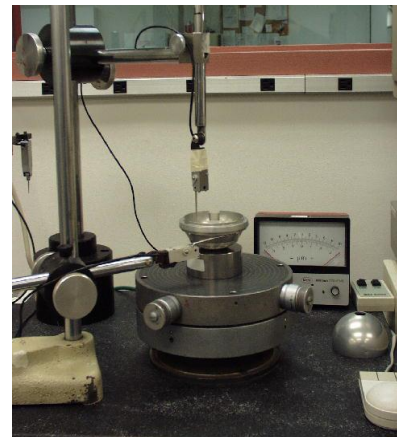
Figure 13 Spherical Bearing under test
